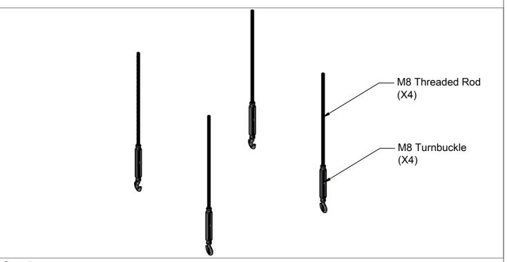
Step 5: Lift up the ATM-470C. Use the hooks at the turnbuckles to hang the ATM-470C at the M8 eye bolt provided.
