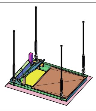
Step 1: Prepare the threaded rods of length (X - 220mm) according to the illustration drawing below. Total of 4 pieces of M8 threaded rods are required.
