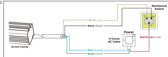
E) Terminate AC cable as shown in figure.
