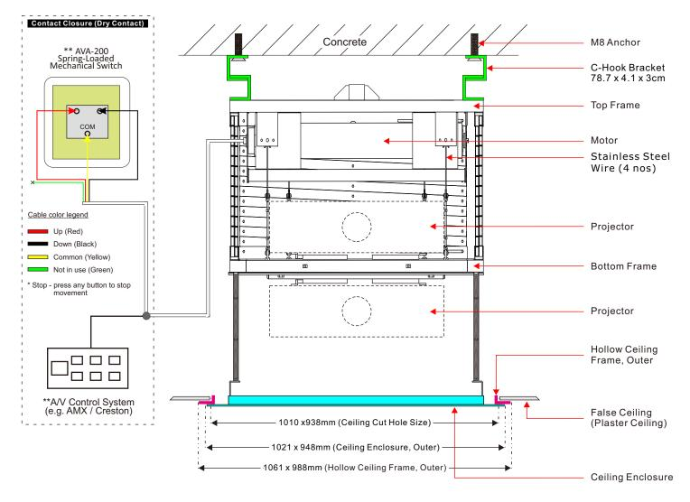
\*\* Momentary Contact closure connection (dry contact, normally open, voltage free). Recommended to set close contact for 1.5sec for best working condition. Any voltage above 3Vdc voltage will damage the motor. Suitable to use with control systems (example: AMX, Crestron, Extron, ..etc) Warranty void if damaged is caused by inappropriate use
